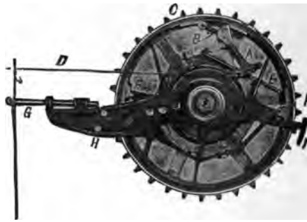
FIG. 387.—The "Duryea" Expanding Break. The two ends of the metal band are separated by the lever, A, and the adjusting screw, B, which is swiveled to the hinge, C. A forward pull on lever, A, through the chain, pull, indicated by D, causes the two ends of the band to be thrust apart and bear against the inner surface of the sprocket. The extension spring, E, normally holds the band away from this friction surface. The two lugs, FF, attached to a spider hung on the axis of the sprocket, take the braking effort from the bottom of the band more into the line of travel. A framework, indicated at H and I, supports a leather guard covering both the chain and sprocket.
